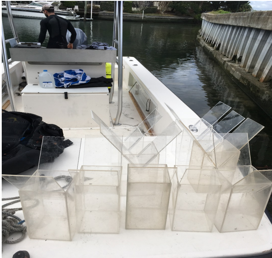
Figure 6. Clear plastic “Breder Traps” for sampling fish communities in shallow waters.
