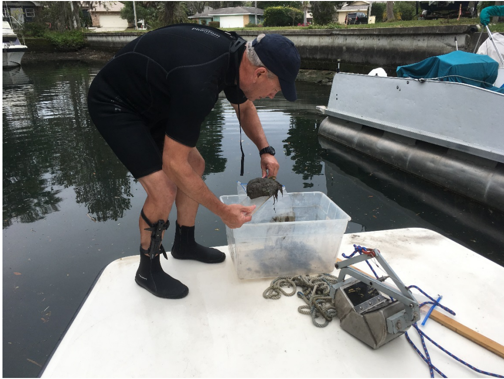
Figure 5. Petite Ponar dredge (lower right) being used to collect replicate sediment samples from restored canal habitat in King’s Bay Area 3.
