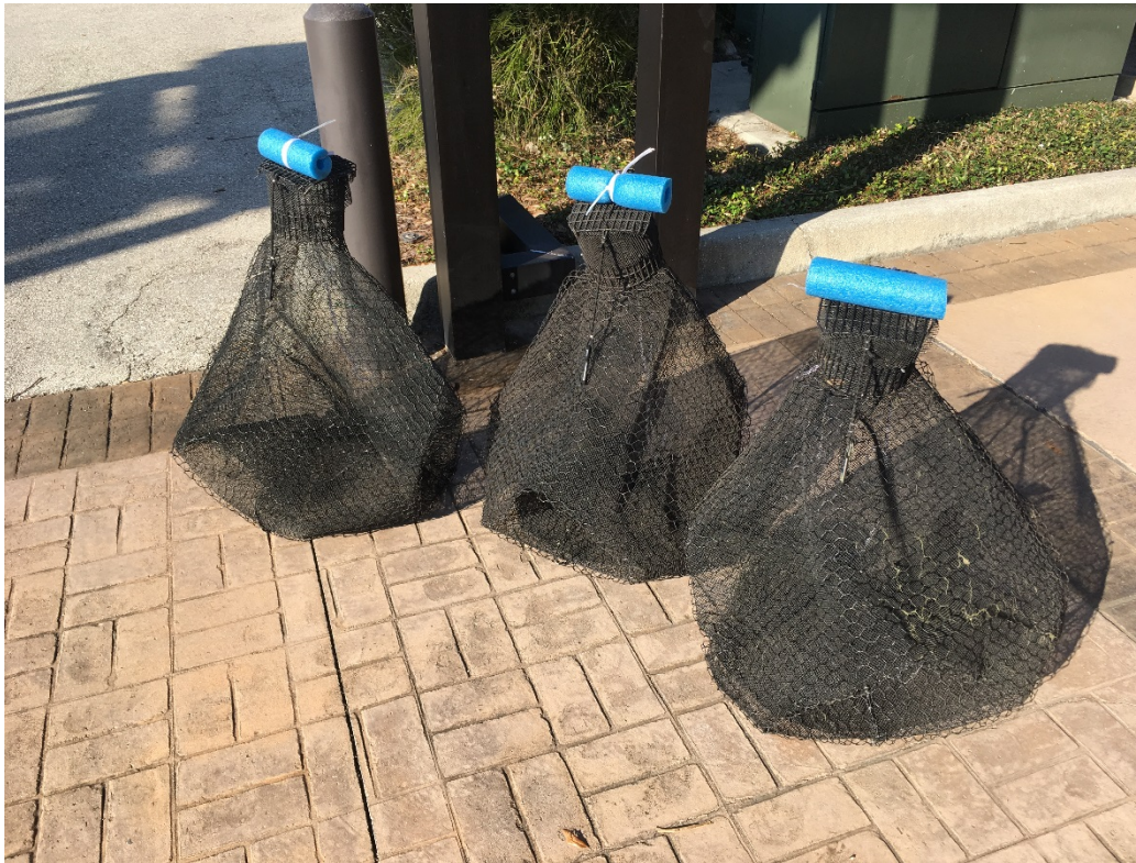
Figure 7. Modified crayfish traps for overnight sampling of fish communities
