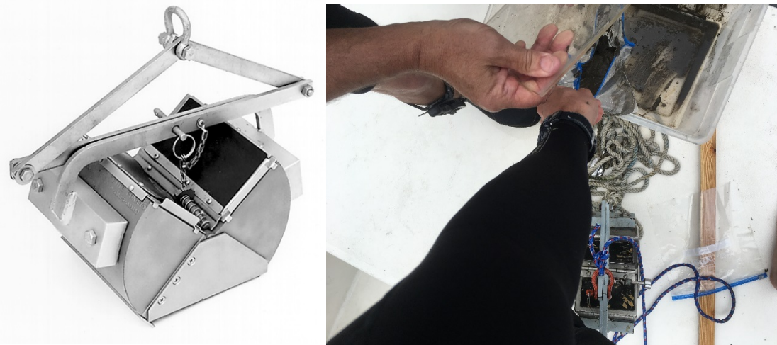
Figure 5. Petite Ponar dredge (left) being used to collect replicate sediment samples (right) from restored canal habitat in King's Bay Phase 1A.
