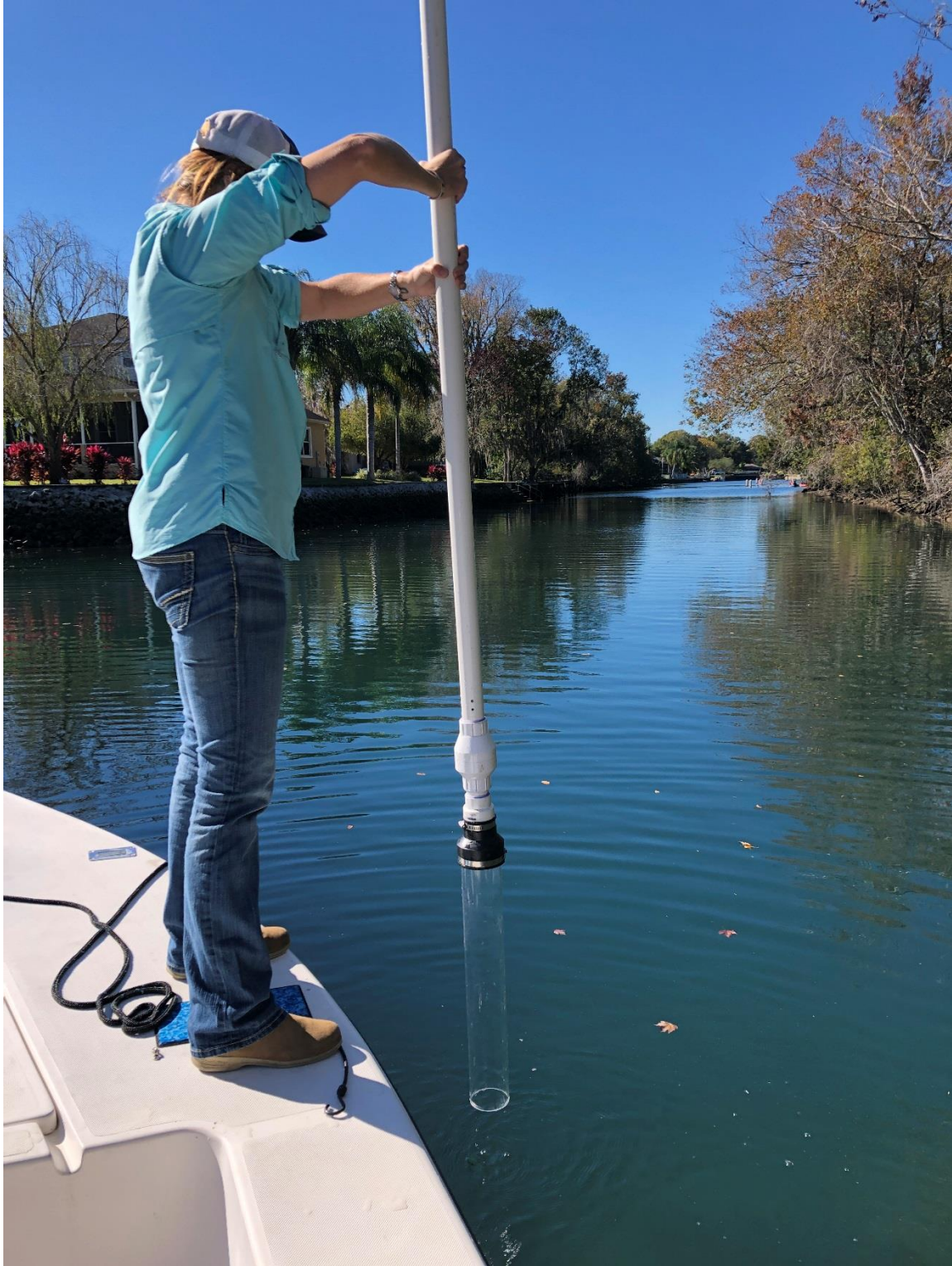
Johnson Engineering ecologist deploying customized core sampler in Canal near Three Sisters Spring, Kings Bay, Citrus County Florida.
