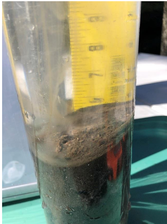
Canal 3; Core Sample 2 with 10.2 cm mud/sand, 2.5 cm clay, and \leq 0.1 cm floc.
