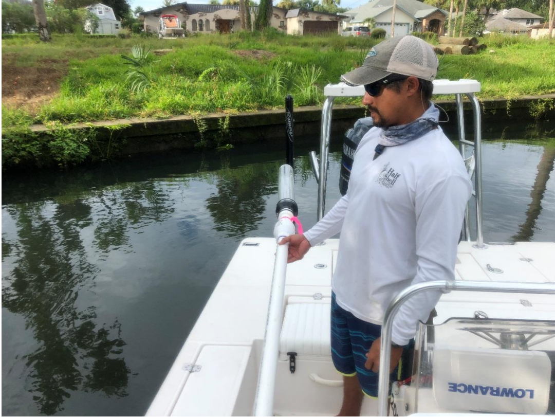
Figure 1. Core sampling device ready to be deployed pre-restoration in Canal 3, August 13, 2018.
