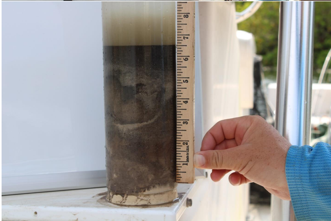
Phase 2-B: Core Sample 2 with 0.3 cm floc and 16.5 cm mud/sand layers.
