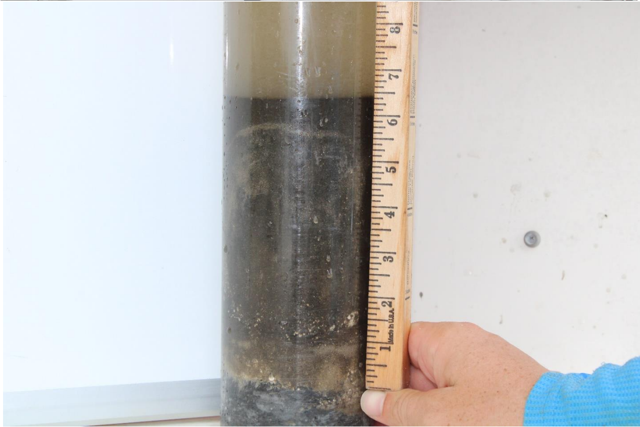
Phase 2-B: Core Sample 5 with 2.3 cm floc and 14.0 cm sand/mud layers with shell.
