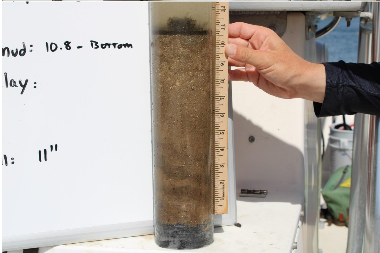
Phase 2-A: Core Sample 3 with 0.5 cm floc and 27.4 cm sand/mud.
