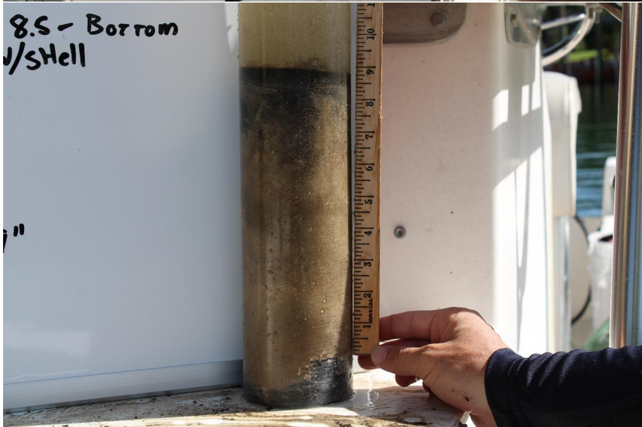
Phase 2-A: Core Sample 1 with 1.0 cm floc and 21.6 cm sand/mud.
