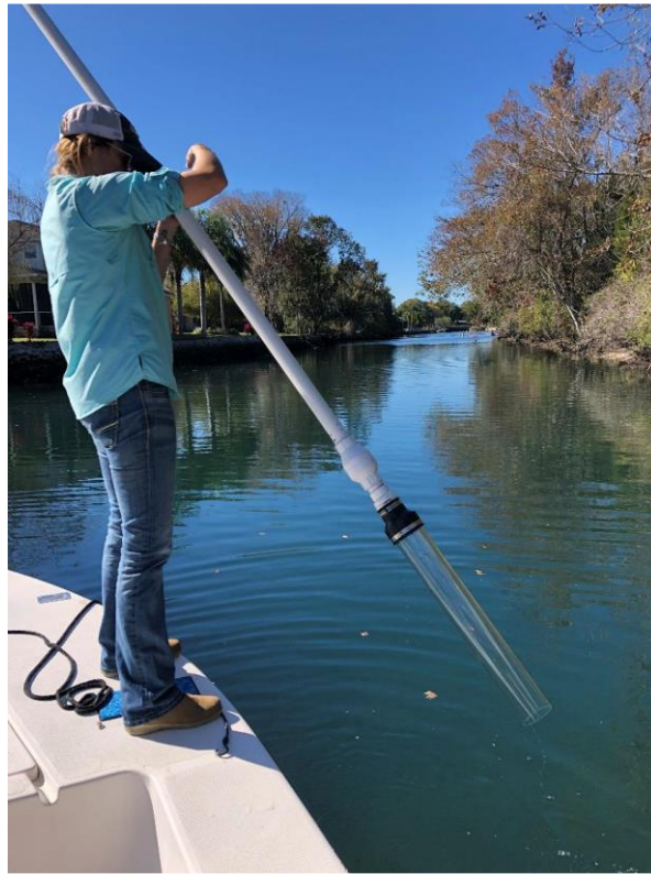
Figure 2. Custom core sampling device used to collect sediment samples for benthic assessment.
