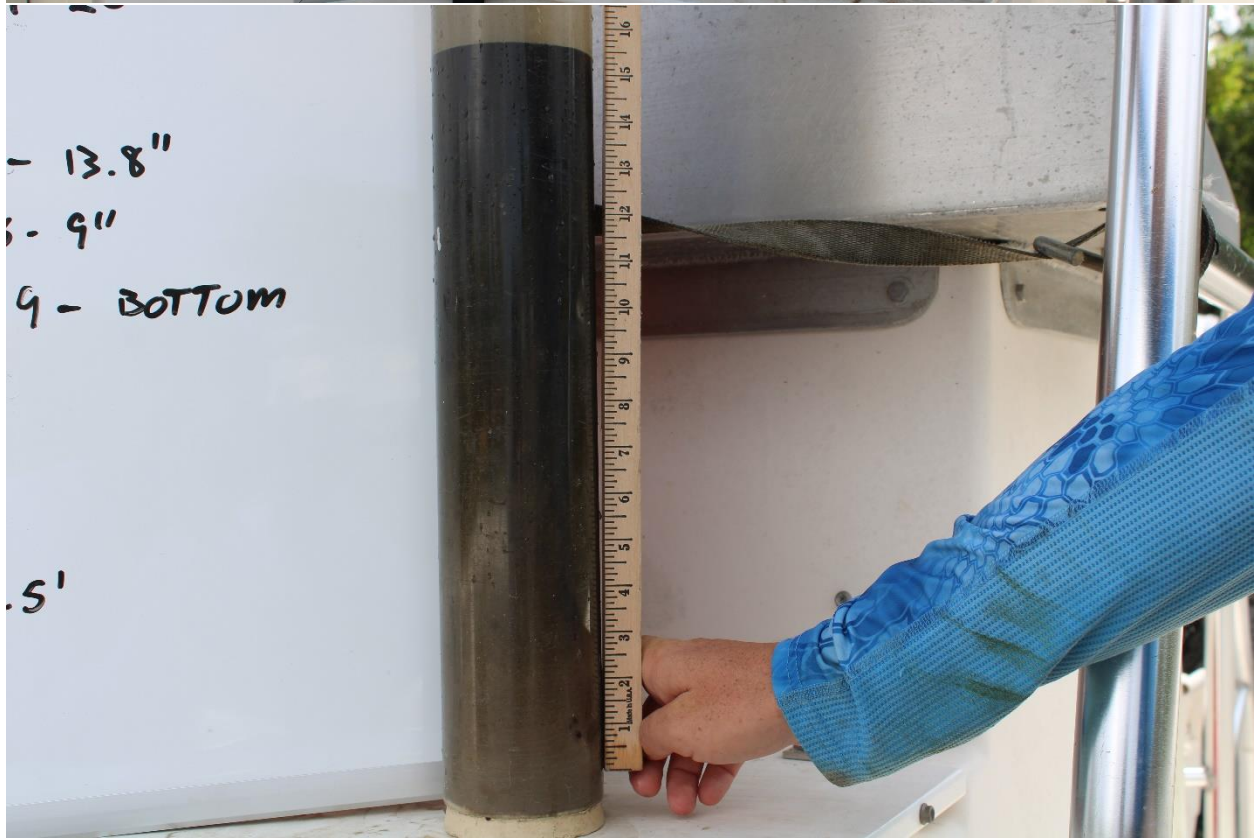
Phase 2-B: Core Sample 3 with 4.3 cm floc and 35.1 cm mud and sand/mud layers.
