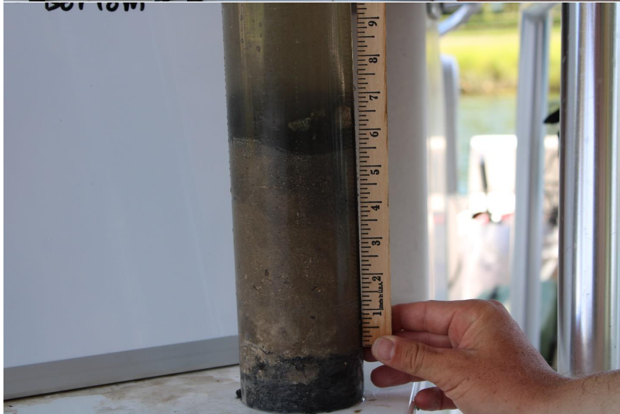
Phase 2-A: Core Sample 5 with 1.3 cm floc and 16.2 cm sand/mud and rock/shell layers.
