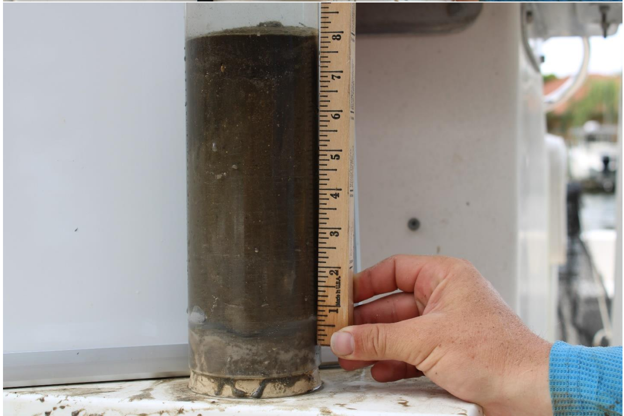
Phase 2-B: Core Sample 4 with 1.0 cm floc and 19.3 cm sand/mud layers.
