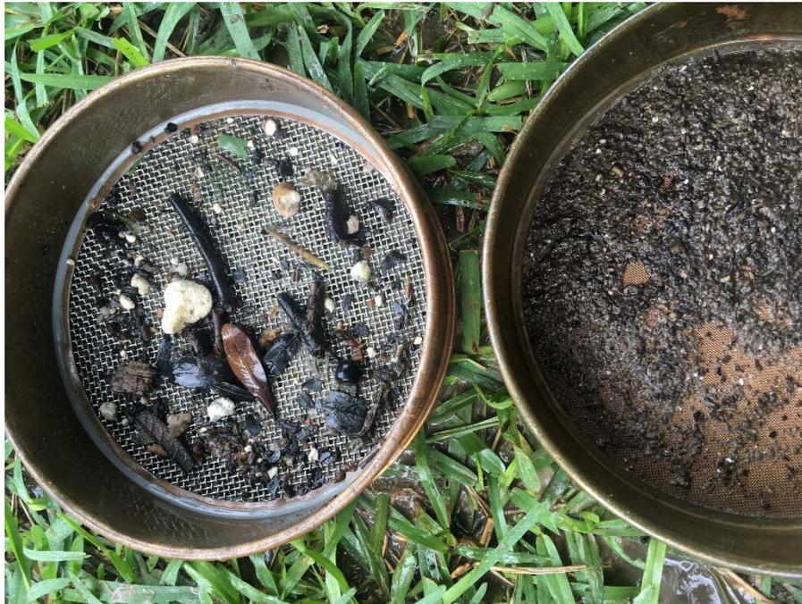
Two standard sieves used to sort petite Ponar benthic samples with sieve #10 (2 mm) on left and sieve #30 (500 micron) on right.
