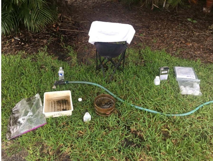
Ponar Sample processing and preservation station using standard sieves to sort benthic macroinvertebrates from sediments and debris.
