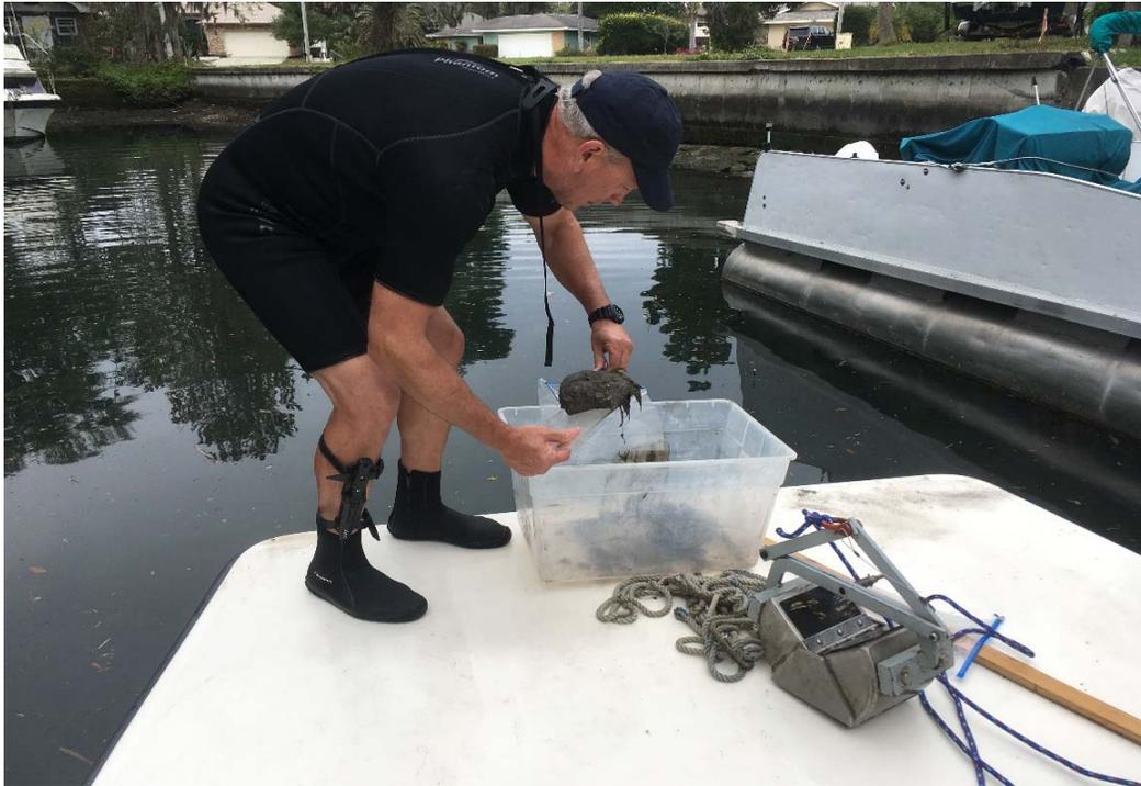
**Figure 5.** Petite Ponar dredge (lower right) being used to collect replicate sediment samples from restored canal habitat in King’s Bay Pilot Project (Area 3).
