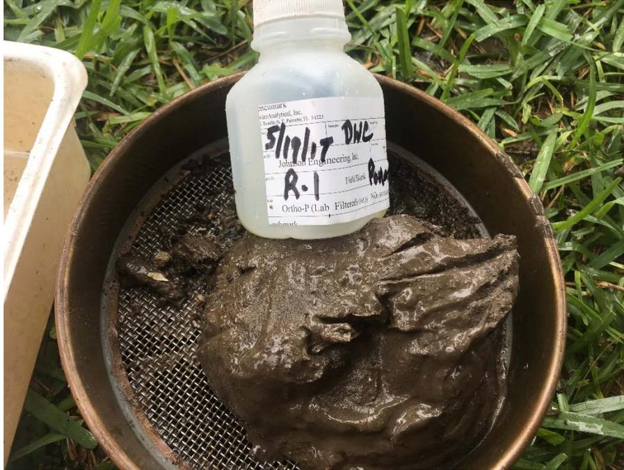
Restored Site Ponar Sample “R-1” showing clay and silt that was not present in other samples collected from the restored canal site.
