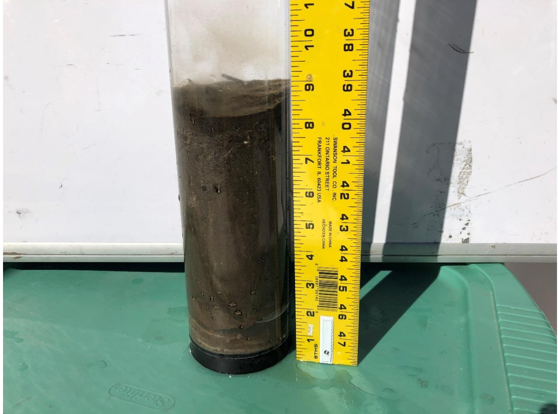
Canal 7: Core sample 4 with 1.9 cm of floc over 19.0 cm of mosly muckl/mud and some sand.
