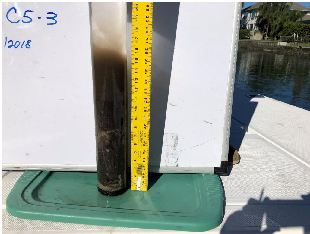
Canal 5: Core sample 3 with 8.9 cm of floc over 19.1 cm of mud/muck and peat.
