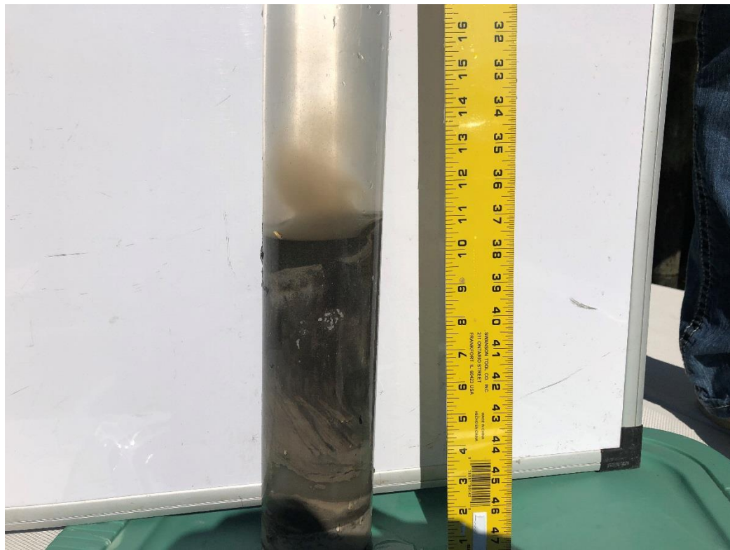
Canal 5: Core sample 1 with 2.0 cm of floc over 2mud/clay and sand layers.
