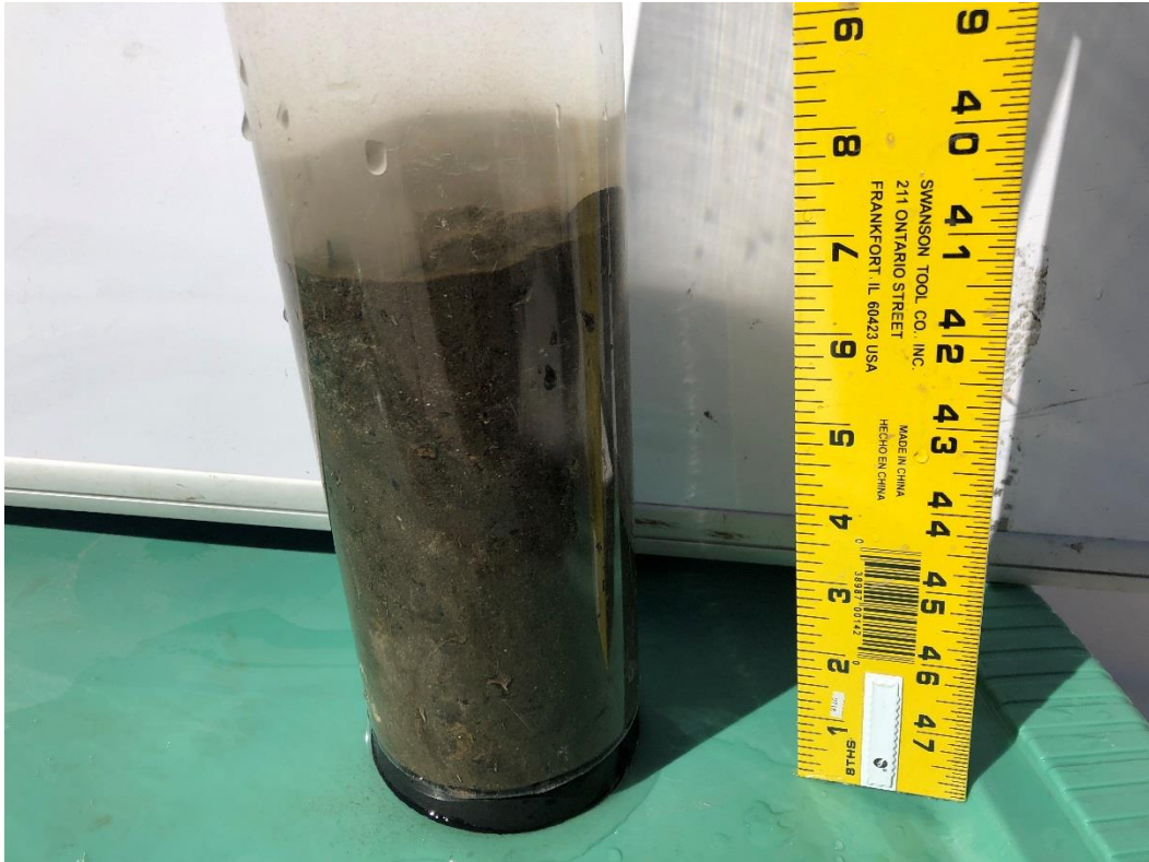
Canal 7: Core Sample 3 with 5.0 cm of floc over 14.0 cm of mostly muck/mud and some sand.
