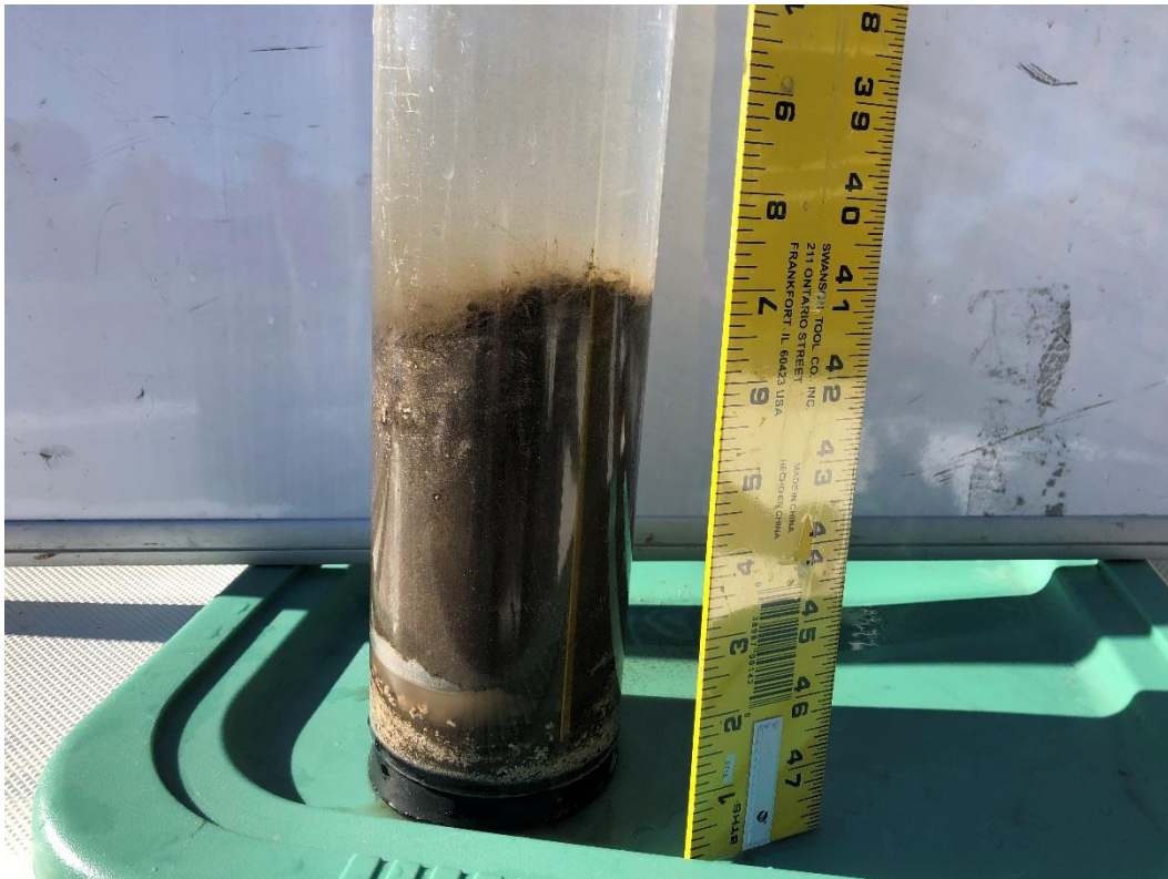
Canal 5: Core sample 5 with 3.8 cm of floc over 13.9 cm of mud/clay and sand layers.
