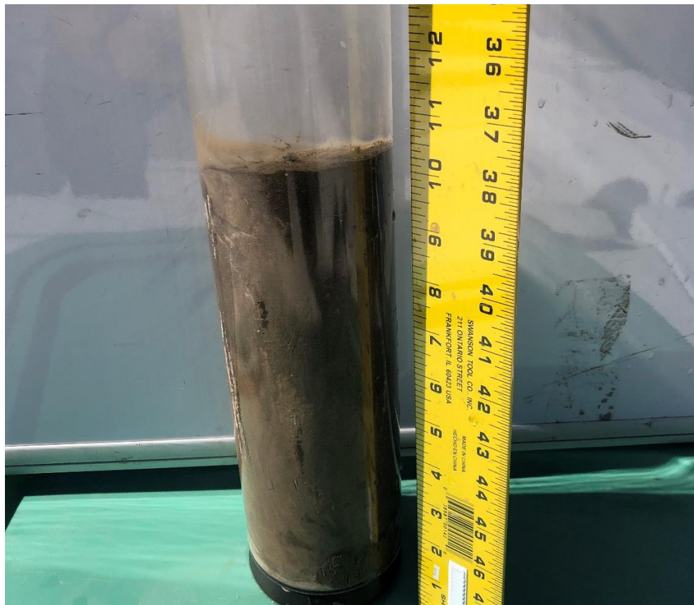
Canal 7: Core sample 2 with 0.3 cm of floc over 26 cm of mud/sand and shell layers.
