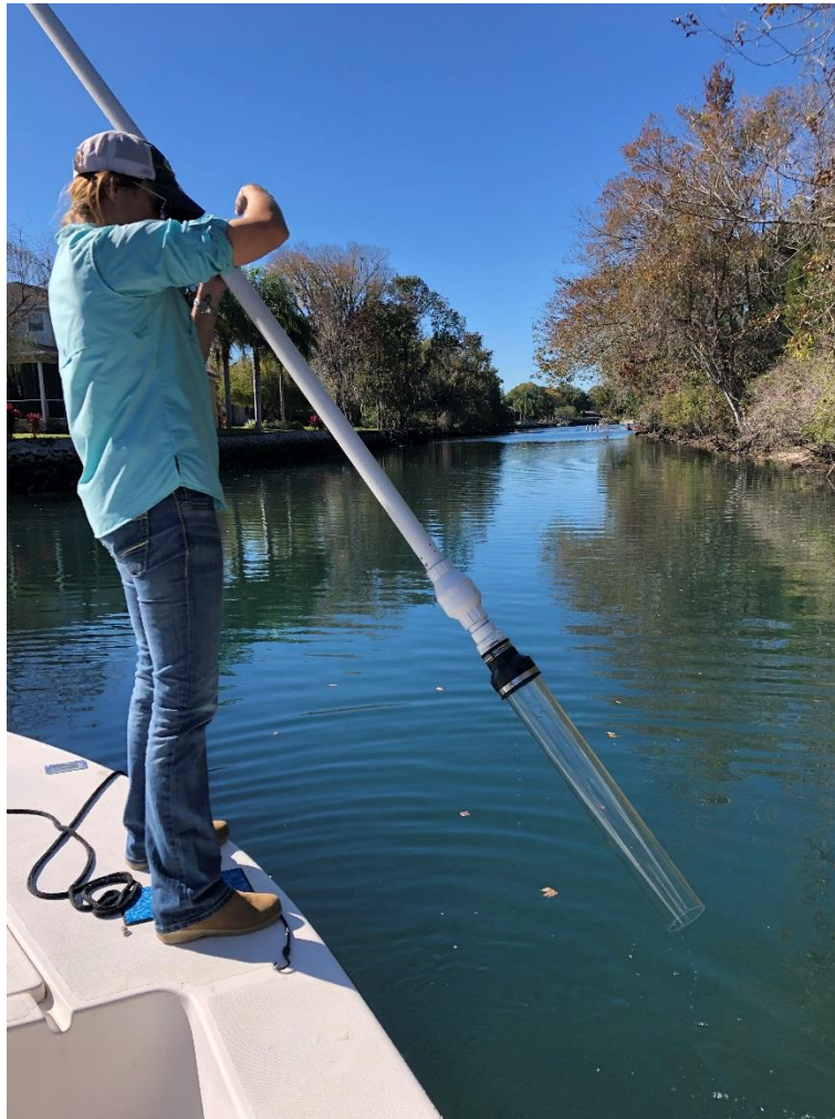
Figure 2. Core sampling device ready to be deployed in Canal 7 on December 6, 2018.
