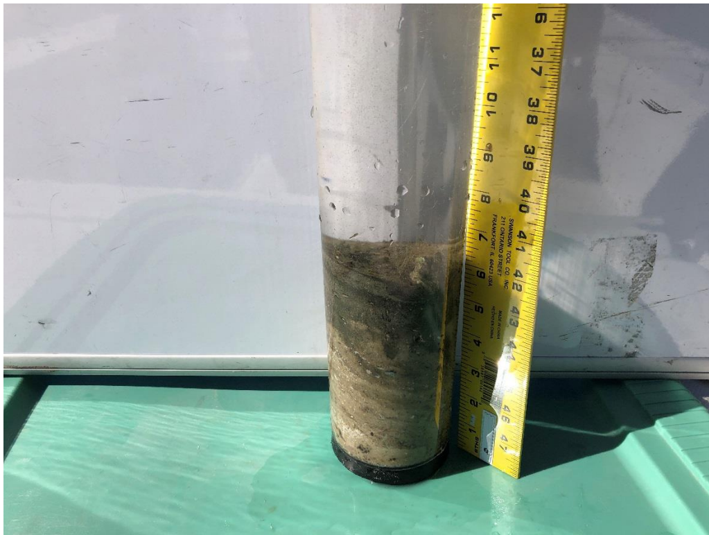
Canal 7: Core sample 5 with 0.7 cm of floc over mud (5.0 cm) and sand/shell (10.2 cm).
