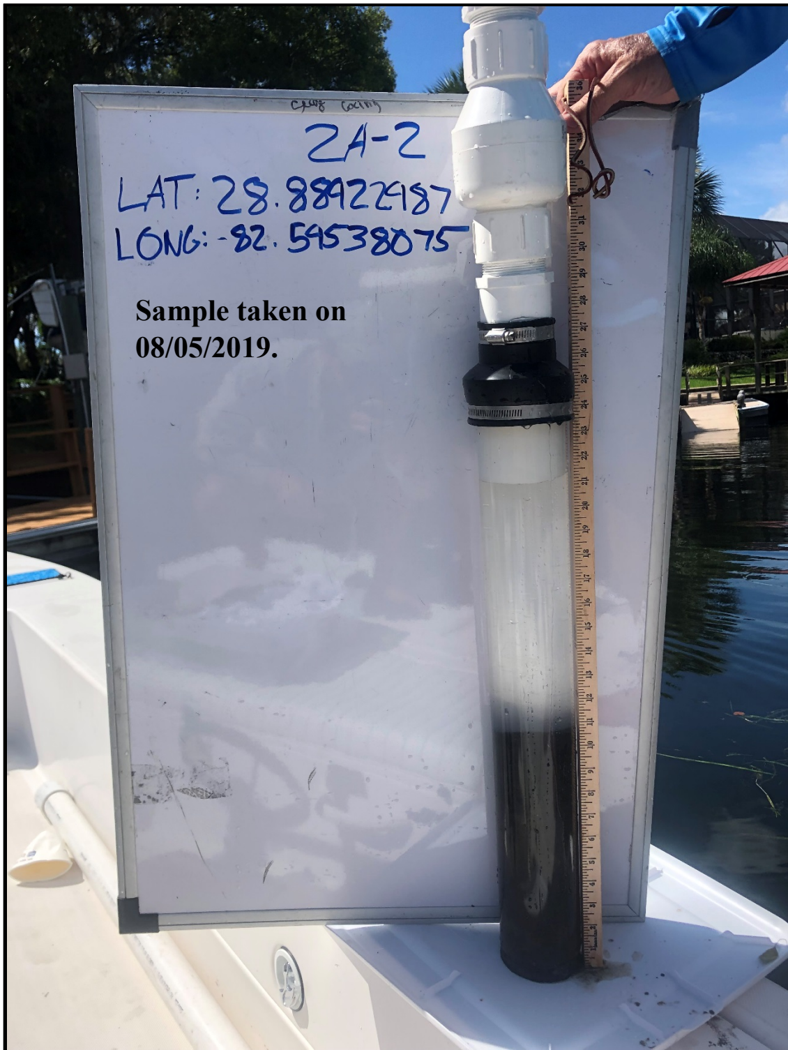
Phase 2A (Canal 2A1) Site 2A-2 – 2.5 cm of floc over 10.2 cm of mud over 12.7 cm of sandy mud.
