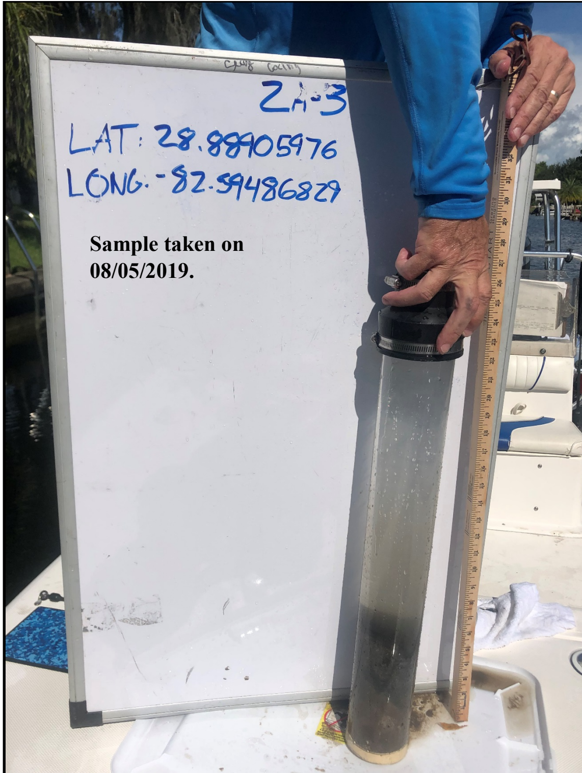
Phase 2A (Canal 2A1) Site 2A-3 – 2.5 cm of floc over 16.5 cm of sandy clay.
