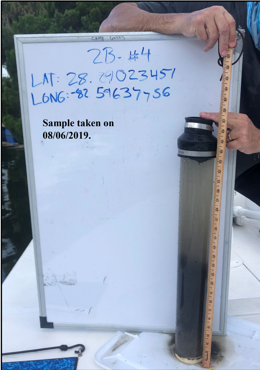
Phase 2B (Canal 2B2) Site 2B-4 –14.0 cm of floc over 5.1 cm of mud over 7.6 cm of sandy mud.
