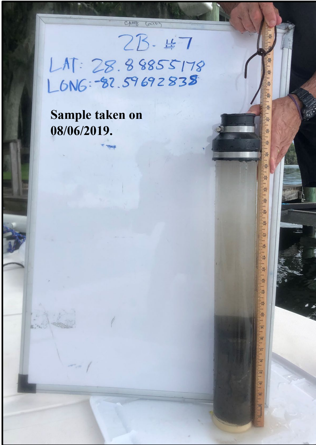
Phase 2B (Canal 2B3) Site 2B-7 – 1.3 cm of floc over 6.4 cm of sandy mud over 15.2 cm of sandy clay.
