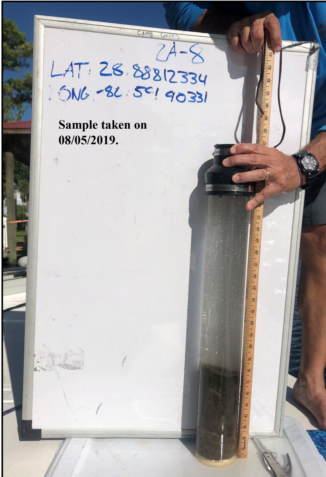
Phase 2A (Canal 2A1) Site 2A-8 – 4.5 cm of floc over 7.0 cm of mud over 10.2 cm of sandy mud.
