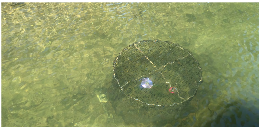
Specially designed, patented exclusion cages designed to protect newly planted tape grass
